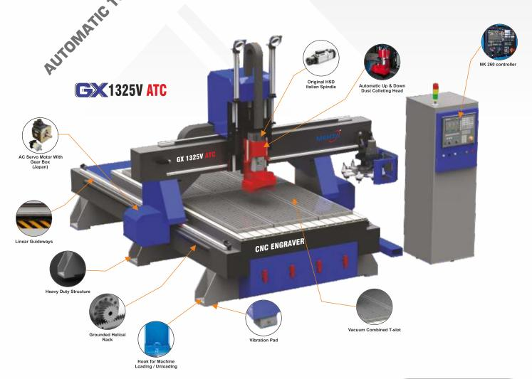
The ATC system includes the HSD spindle, a pneumatically assisted Z axis, eight-position tool bank, fixed-position Z-zero plate, chuck holder, pneumatically operated dust collacting head.
